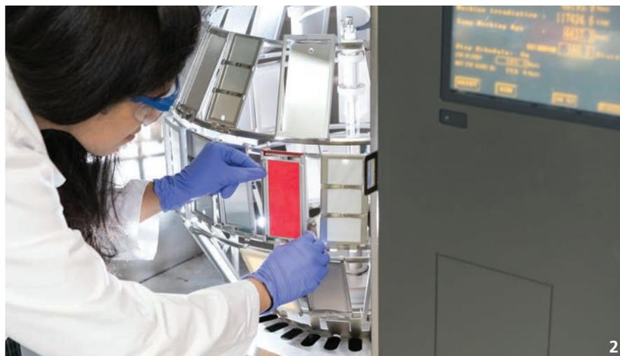
1 © Fraunhofer USA, Fraunhofer CSE – climate chamber for photovoltaic (PV) module and material testing
