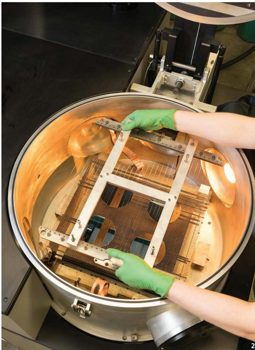
1 © Fraunhofer USA, Fraunhofer CCD engineers working in CCD's cleanroom loading a PVD sputter system
